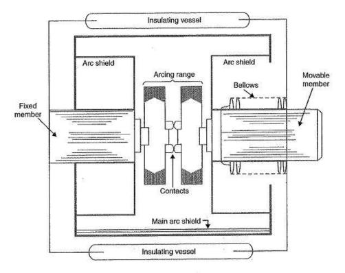
**Working**: When the breaker operates, the moving contact separates from the fixed contact and an arc is struck between the contacts. The production of arc is due to the ionisation of metal ions and depends very much upon the material of contacts.
