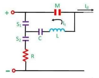
For interrupting main circuit current  $I_d$ , the operating mechanism open contact  $S_2$  and closes contact  $S_1$ . This indicates discharge of capacitor C through inductance L, main contact M and auxiliary contact  $S_1$  setting up an oscillatory current shown in the figure below. Thus, artificial current zeros are created, and the circuit breaker main contact M is opened at a current zero. After that, contact  $S_1$  is opened, and contact  $S_2$  is closed.
