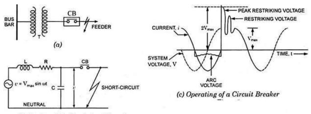
(b) Fault and its Equivalent Circuit
